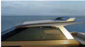
rotating T-top transforming Bimini into Hardtop and vice versa
