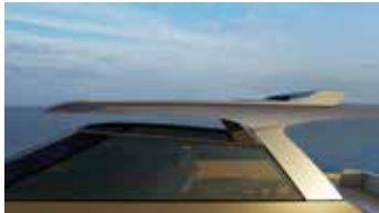
rotating T-top transforming Bimini into Hardtop and vice versa
